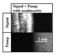
FIG. 4. Photographs of each of the locked beams of Fig. 3(b) monitored separately. The overlap between the beams remains unchanged throughout propagation.
