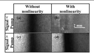
FIG. 3. Photographs of both beams at the output face of the crystal, displaying (a),(c) separated shock fronts during linear propagation, (b) locked shock waves when the signal is weaker than the pump  $(I_b > I_a)$ , and (d) increased separation when the signal is stronger than the pump  $(I_b < I_a)$ .
