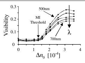
FIG. 3. Visibility as a function of the nonlinearity strength. Different curves correspond to different wavelengths (temporal frequencies).
