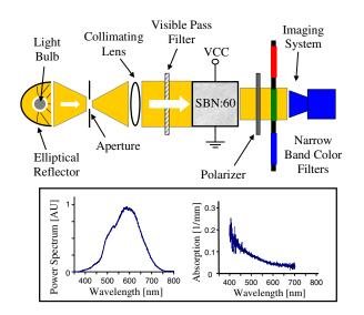
FIG. 1 (color online). A sketch of the experimental setup. The inset shows the temporal spectrum of the light at the input face of the crystal (left) and the crystal absorption (right).
