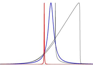
Fig. 2. (2.4 MB) Movie of the cavity wavelength response (<u>6.6 MB version</u>). The scanningpump (red) induces thermal drift of the resonant lineshape (blue). The intersection point between the pump line and the cavity Lorentzian draws the hysteretic absorption (black). Parameters here are identical to the parameters in Fig. 1(b). The movie is in slow motion as each scan cycle truly takes 80 *ms*
