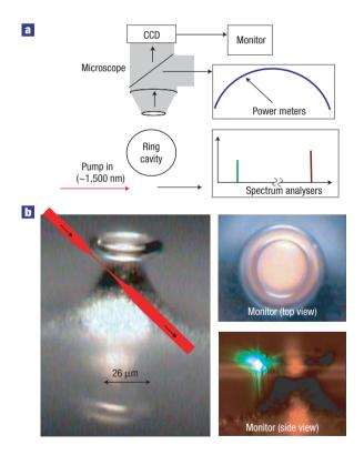
**Figure 1 Experimental set-up. a**, Infrared pump (of 300 kHz bandwidth) evanescently coupled to a microring cavity by a tapered fibre, generating visible TH emission. The TH emission is monitored by a camera, detector and a spectrum analyser. **b**, Left: The tapered fibre via which the pump is evanescently coupled into the ring cavity. Right: Top and side view of the cavity; TH power is visible in the side view.
