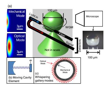
FIG. 1 (color online). (a) Left: Cross sectional views of the calculated mechanical and optical modes (stress and electric fields). Right: Experimental setup. (b) Illustration of a moving cavity element as in other photonic MEMS. (c) Illustration of our WGM cavity where the acoustical and optical modes are circumferentially circulating.
