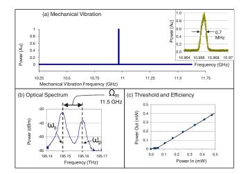
FIG. 2 (color online). Experimental results. (a) Vibration readout from an electrical spectrum analyzer which is connected to a photodetector. (b) Readout from the optical spectrum analyzer showing both the Stokes line and the residual scattering of the pump, (c) Power out vs power in.
