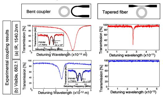
Fig. 2. Comparison between tapered-fiber coupler and bent taper coupler, experimental results. (a) Coupling at IR (1540.2nm). (b) Coupling at visible (682.1nm). Insets describe the transmission in the under-coupled regime and are used for measuring the resonance width. The linewidth is narrow enough to resolve a fine splitting between the clockwise and counter clockwise modes.
