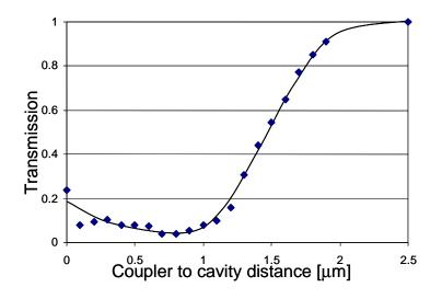
Fig. 4. Experimental measurement of the bent-coupler transmission Vs. coupling distance (squares); the line is a guide for the eye. Cavity external diameter is  $32 \ \mu m$  with minor diameter of 6  $\mu m$ , coupler outer diameter is  $37 \ \mu m$  with minor diameter  $3.5 \ \mu m$ . Optical quality factor is 22 million and wavelength is 1542.4 nm.
